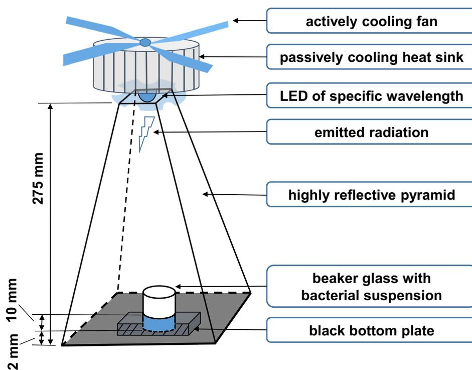
**Figure 2.** Schematic irradiation setup for exposure experiments with different LED wavelengths. Multiple reflection inside of the pyramid leads to homogenous irradiation in the sample area and black bottom plate ensures exclusive irradiation from above as measured with power meter.
