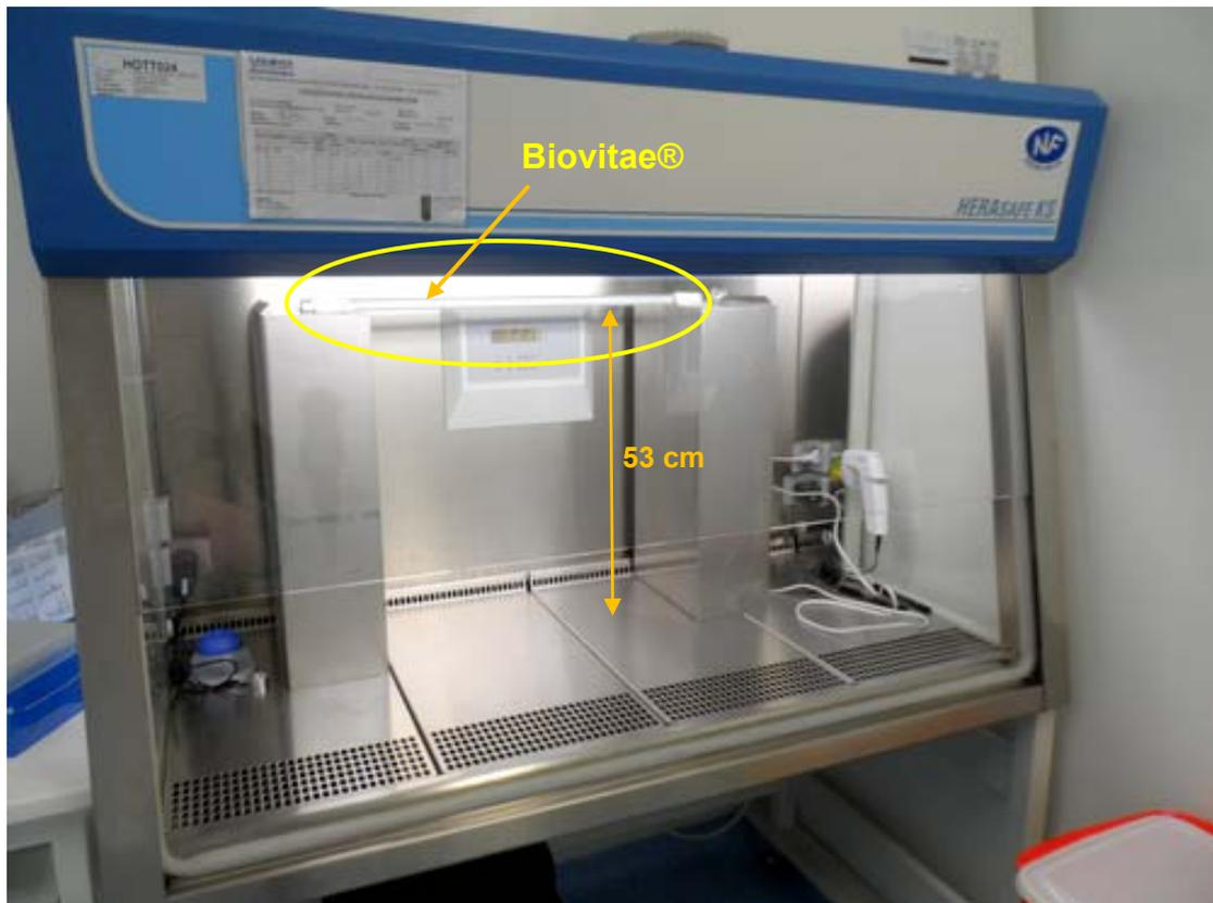
**Fig 2:** Biovitae® lamp installed in a BSC II of the BSL3 laboratory with a height of 53 cm from the work surface.
